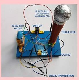
The high voltages cause the air around the tip of the tesla coil to ionize making plasma of lighting up a CFL bulb. A simple tesla coil can be made by using a transistor if have a battery as a power source, the transistor is a high-speed switching device that mimics the direct current to form a sort of alternating current by turning on and off the power supply quickly to form a wave like voltage change similar to that of a pure sine wave of alternating current
